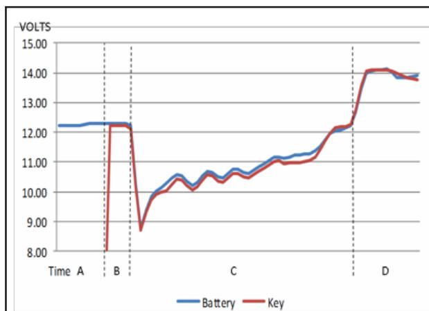
**Figure 2: Voltages for Electrical System Four Operating Modes**
