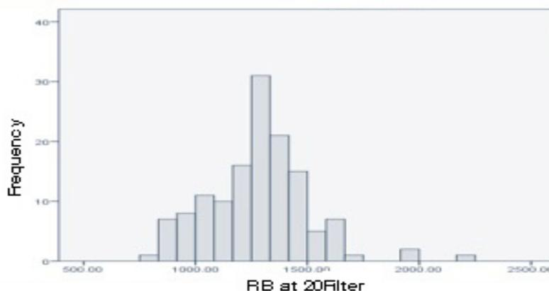
**Figure 4: Battery Internal Resistance Corrected to 20°C**
