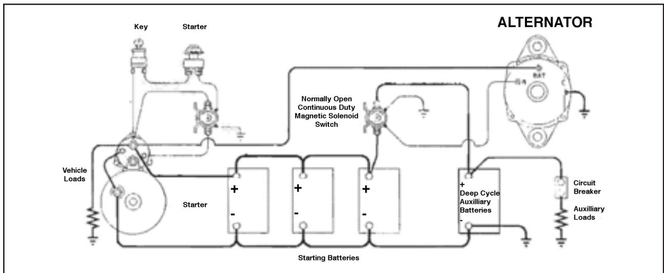
**Figure 1: Typical Primary Electrical System**
