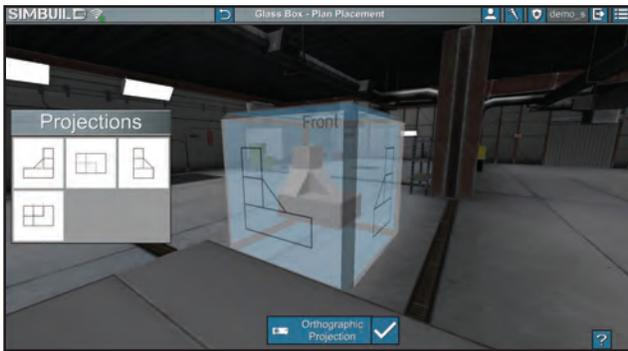
**Figure 7: Print Reading and Orthographic Projections Taught Through a “Glass Box” Activity in SimBuild™ Industrial.**
